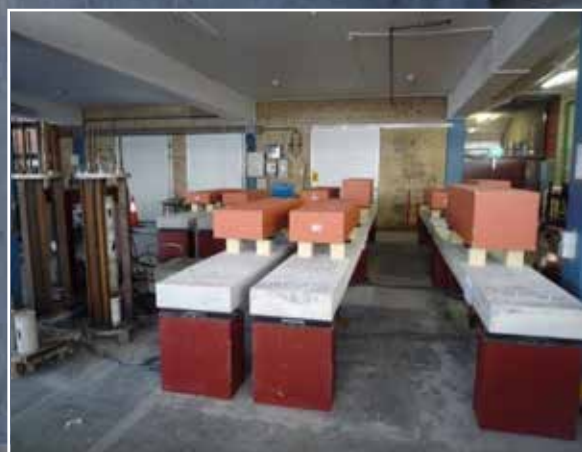
Figure 1: Slab specimens under sustained loads
