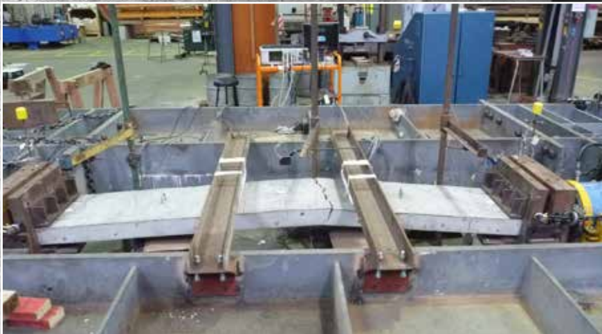
Left - Figure. 1: Testing of panels for time effects
