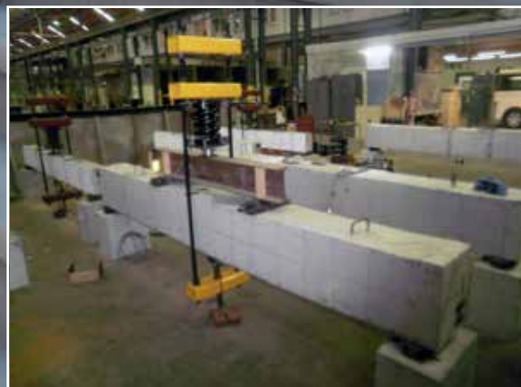
Figure 2: Beam specimens under sustained loads
