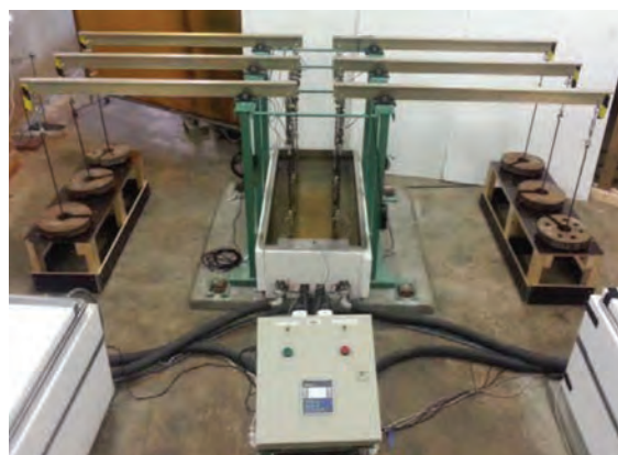
Figure 1: Thermal cycle apparatus
