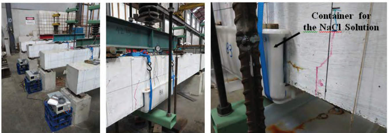
Figure 1 - Arrangement of testing setup for accelerated corrosion
